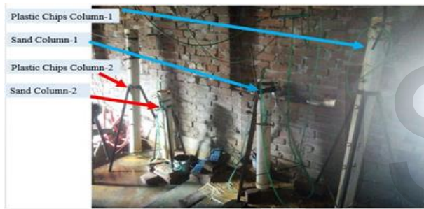
Figure-7. Column set up at location B
